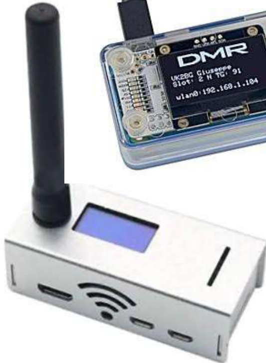
Common MMDVM Hotspot with Raspberry Pi W with small display
