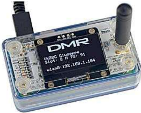
Zum Radio with Raspberry Pi W with display
